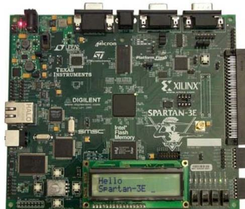
The Xilinx Spartan-3E Starter Board ADC outputs 14-bit two's complement binary data and the DAC requires 12-bit straight binary data. The conversion is accomplished by complementing the MSB of the ADC output (bit 13) as the sign bit. The twelve MSBs of the ADC output (bit 13 through bit 2) are outputted to the DAC. Since the PGA inverts the analog input signal, the resulting straight binary data is complemented for comparison of the analog input and output signals on an oscilloscope.
